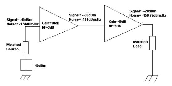
For above example both amplifiers has 10dB gain and NF=3dB.
