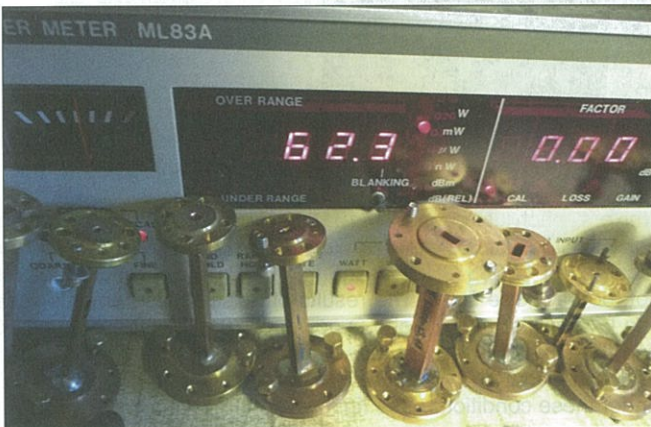
Fig. 6: Output power measurement of the 47 GHz transverter using a homemade 6 dB attenuator
