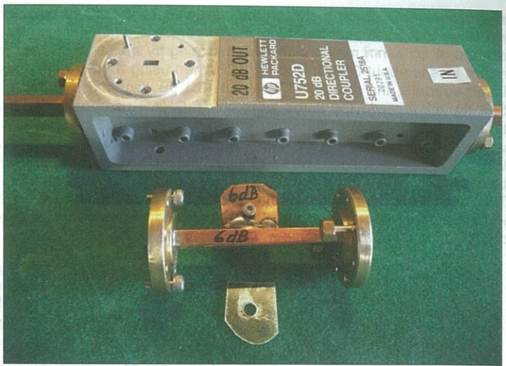
Fig. 3: 47 GHz coupler and homemade 6 dB WR19 attenuator
