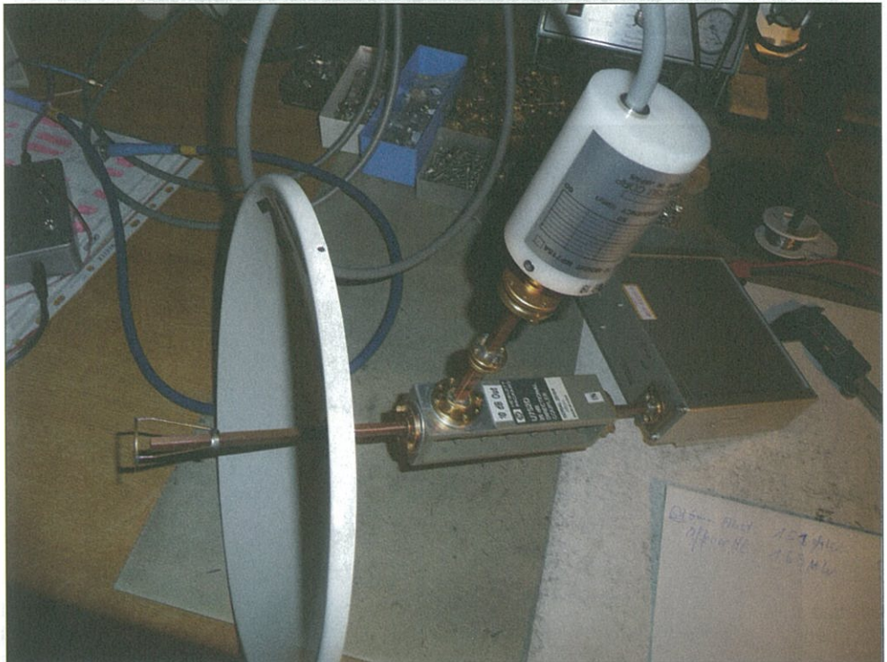
Fig. 10: 25 cm parabolic dish from Procom with WR19 Cassegrain feed for 47 GHz
